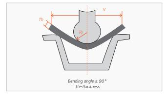
**The bending force** depends on UTS plate thickness, bended length and die opening V. Indicative values, for die opening V = 12th (V bending)
