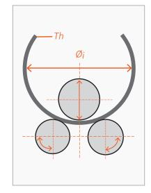
**Creusabro**° **4800** can be hot formed at a temperature of 450 - 500°C (840 - 930°F) without any further heat treatment. At this temperature the force necessary to deform the plate will be lower than at room temperature, and the deformation capability of the steel will be higher (smaller forming radius).
